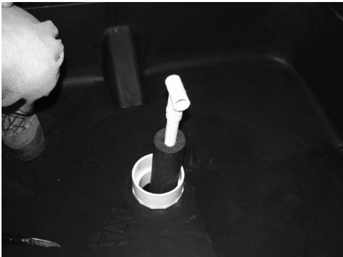
Step 11 Make sure the fitting is straight across and runs parallel with the sides of the tank. It must be straight or the floats will hit on the underside of the lid.
