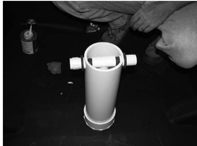
Step 16 Tighten both 3/4" (1.90cm) fittings.
