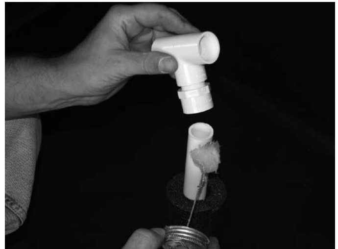
Step 10 After the fitting is tightened into the "T" fitting, apply PVC cement to the \frac{3}{4} " (1.90cm) pipe and install the "T" assembly.
