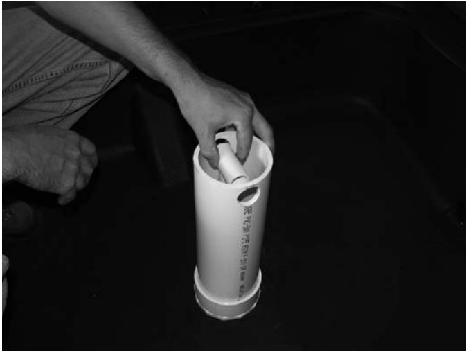
Step 13 Push the 4" (10.16cm) pipe into the lower fitting and align quickly with the "T" fitting so the holes line up with the "T" fittings threaded ends.
