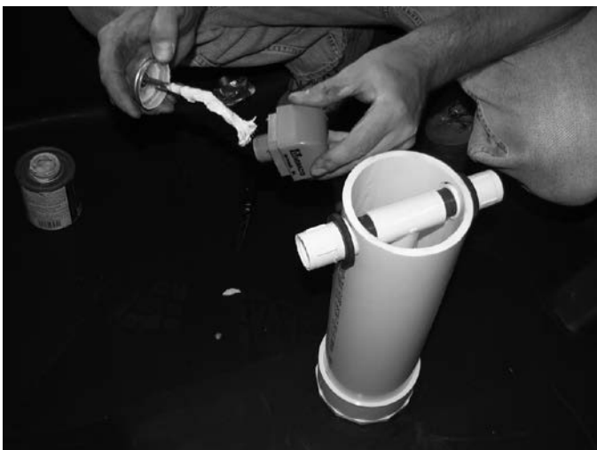
Step 17 Apply pipe dope or teflon tape to the threads on the valve.
